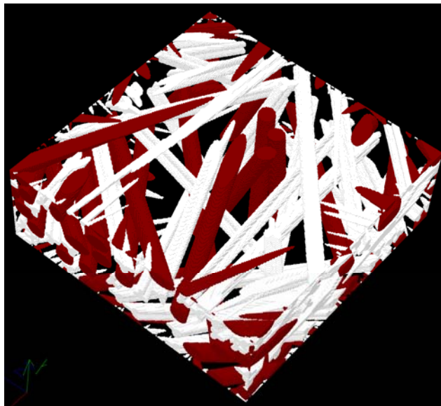
Figure 2: An example of a bi-component fiber-web made up of fibers with circular (red) and trilobal (white) cross-sections. Both components have equal mass fractions.
